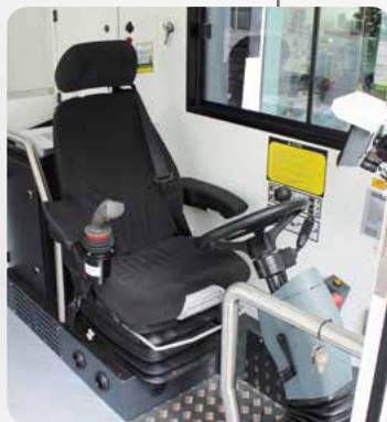
Driver's stand with air suspension comfort seat, joystick and colour touchscreen
