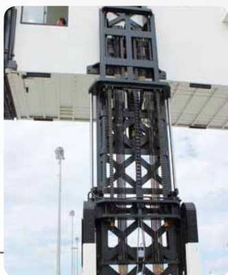
Triplex lift mast – all load-bearing components with a tenfold margin of safety
