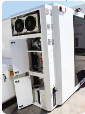
strong auxiliary heating system and AC for continuous operation
