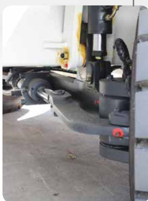
Robust sideloader steering system with almost 90° steering angle
